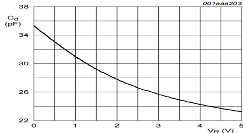
Fig. 5. Diode capacitance as a function of reverse voltage; typical values
