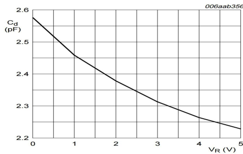
Fig 2. Diode capacitance as a function of reverse voltage; typical values
