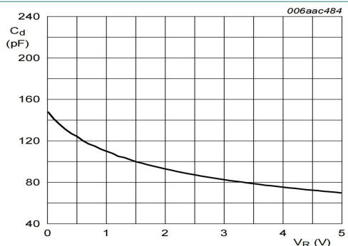
Fig. 5. Diode capacitance as a function of reverse voltage; typical values
